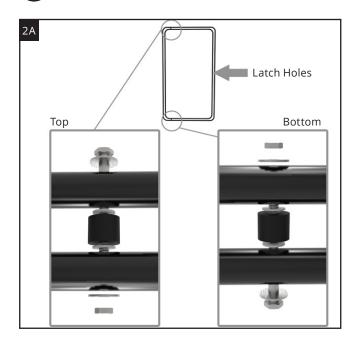
**2A.** Install the hinge hardware as shown for the top and bottom of the gate. Please note: The two black spacers go between the Gate (inner) and Frame (outer).
